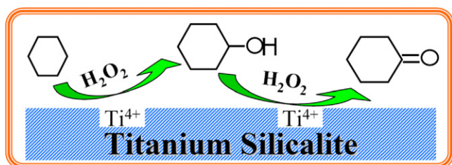
Scheme 3. Simplified scheme of the proposed reaction mechanism of cyclohexane oxidation over titanium silicalites with \text{H}_2\text{O}_2 as oxidant.
